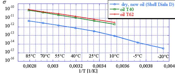
**Figure 2:** Thermal dependency of the specific conductivity of mineral oils with a moisture content of approx. 11ppm (Arrhenius representation)
