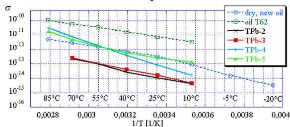
**Figure 5:** Thermal dependency of the specific conductivity of the material samples TPb-1-5 and oils
