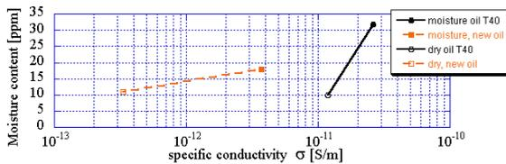
**Figure 3:** Specific conductivity in dependence of the moisture content of new mineral oil and the oil sample T40 at a temperature of 40°C
