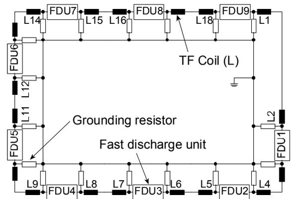
Fig. 2: Simplified analogue circuit of the ITER coil system during a fast discharge (power supply already disconnected). The network model itself is more comprehensive e. g. it includes instrumentation cables and internal elements of the FDUs.
