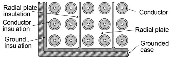
Fig. 1.: Part of the cross section of an ITER TF coil showing the three different types of the electrical insulation.
