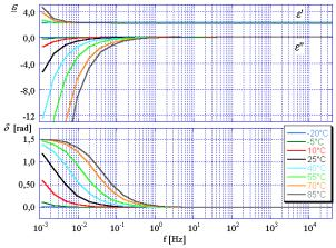
Figure 1: Curve run of the complex permittivity of new mineral oil in different temperatures
