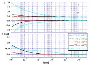
Figure 4: Curve run of the complex permittivity of transformer boards TPb-1-5 at 40°C
