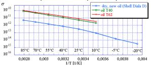
**Figure 2:** Thermal dependency of the specific conductivity of mineral oils with a moisture content of approx. 11ppm (Arrhenius representation)
