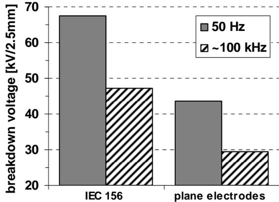
Fig. 3: Comparison of different electrode shapes
