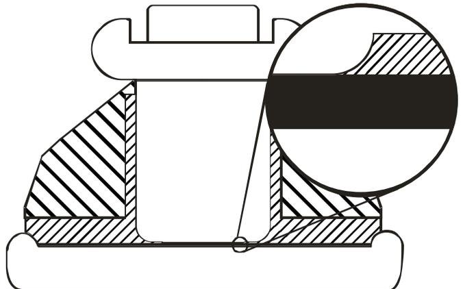
Fig. 2: Test vessel for solid dielectrics
