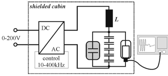
Fig. 1: Setup of the resonance circuit
