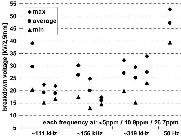
Fig. 4: High frequency breakdown tests for mineral transformer-oil
