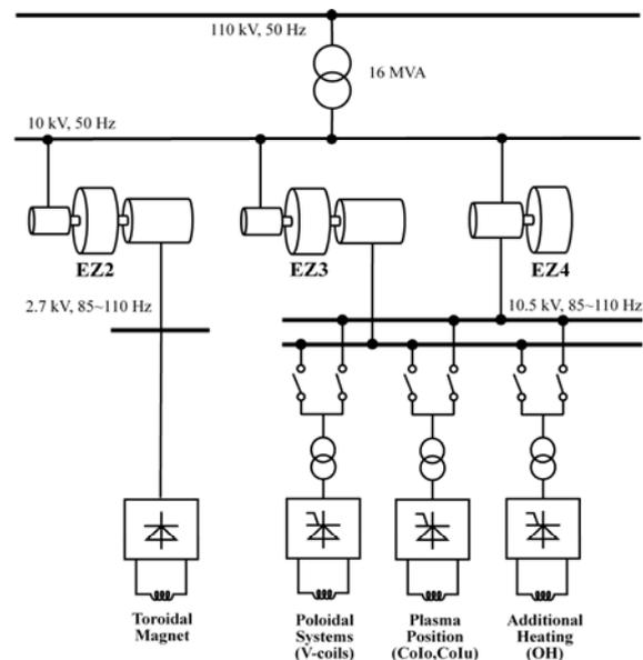
Fig. 1. Structure of the IPP experimental power supply
