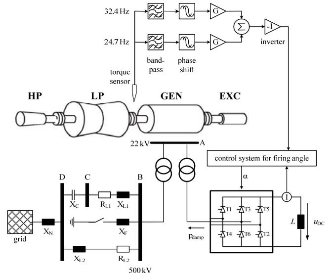
Fig. 7. Electrical network representation of the IEEE Second Benchmark Model for SSR simulations and active damping circuit for a turbine generator (with an extended control module for multi-mass system)
