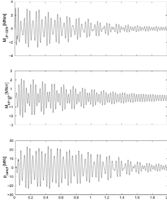
Fig. 9. Active damping of SSR case shown in Fig. 8 (damping circuit configuration shown in Fig. 7)
