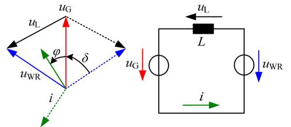
Fig. 11 Monophasic equivalent network of the system with vector diagram
