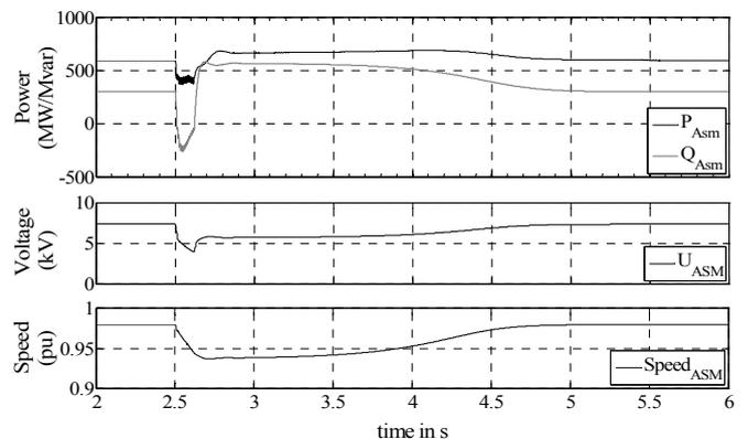
Fig. 7. Fault applied and no MSC in service – voltage and speed
