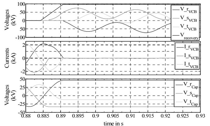
Fig. 3. Voltages and currents of the VCB and voltages across the capacitors
