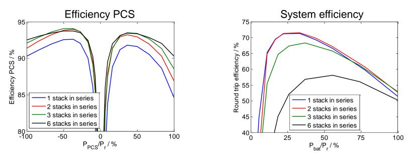
In this case: Series connection of two stacks is optimal.
