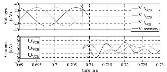
Fig. 4. Voltages and currents of the VCB while connecting a MSC
