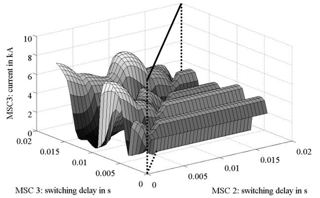
Fig. 9. Current as a function of the delayed switching of MSC 2 and 3
