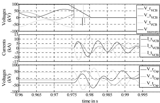
Fig. 5. Voltages and currents while connecting a pre-charged MSC
