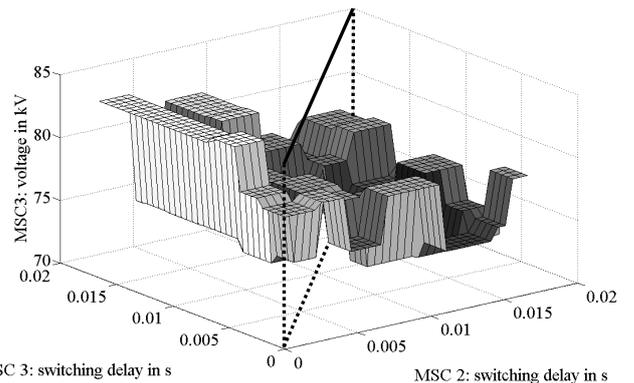
Fig. 10. Voltage as a function of the delayed switching of MSC 2 and 3
