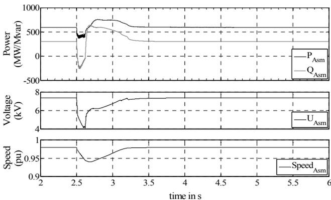
Fig. 8. Fault applied and all MSCs in service – voltage and speed
