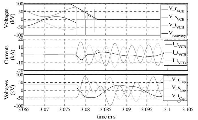
Fig. 6. Voltages and currents while connecting a pre-charged MSC
