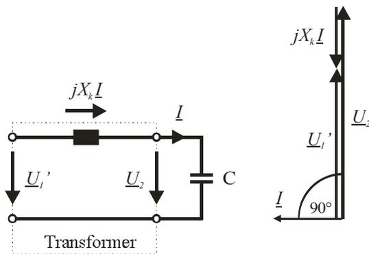
Fig. 1. Capacitive voltage rise at a transformer [8]
